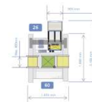
SM481PLUS : The spindle and fiducial camera center recognize two trays (in the width direction)
