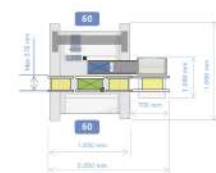
SM481PLUS : The spindle and fiducial camera center recognize two trays (in the width direction)
