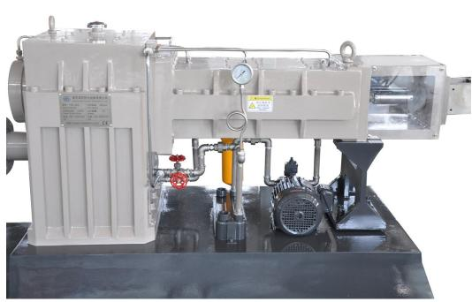
5) Processing section Description Screw barrel
