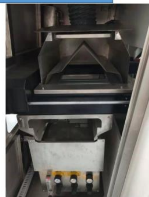
Mountain-shaped Design Flux Recycle
