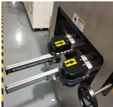
Coneyor Width ajustable, PCB Width: 50-350mm
