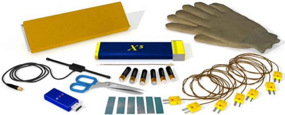
X<sup>5</sup> is KIC's compact, powerful new generation of thermal profilers. The profiler is the data acquisition tool and a component of KIC's thermal process management systems. It physically moves through the thermal process, capturing the temperature and time information that KIC software uses to create a thermal profile.
