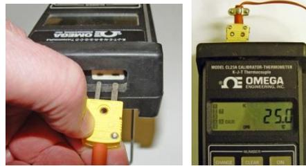
5. Turn on the power to the thermocouple simulator, and set the output value to 25°C (77°F).
