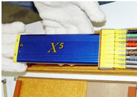
6. Place the profiler in front of a fan or other cooling station arrangement.
