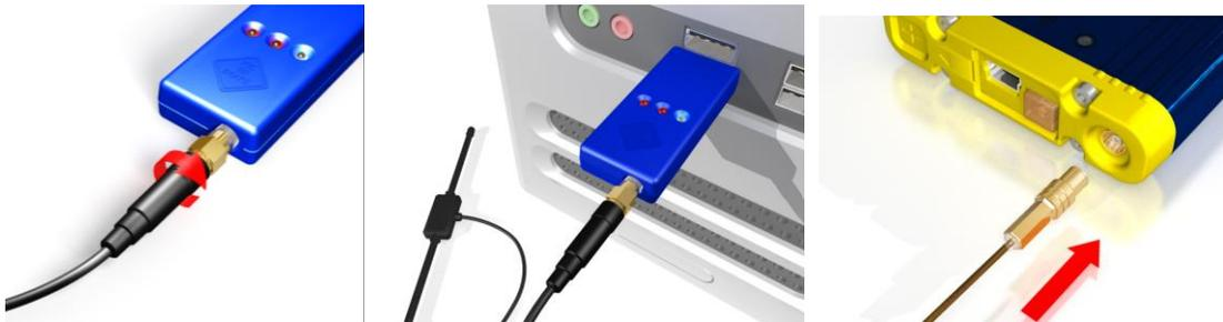
*When you connect the base station, Windows recognizes the USB device, and the Found New Hardware Wizard screen appears.*
