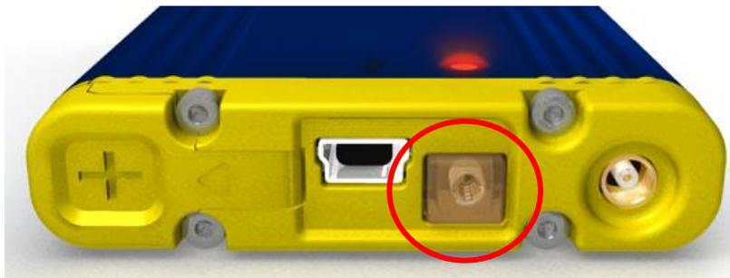
**Power Off** – Press/hold the amber colored On/Off button for 1 second (located at the back of the X<sup>5</sup>). When the power is turned off, the LED indicators will also be off.
