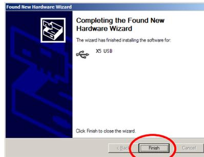
**Note:** The *Found New Hardware Wizard* USB driver installation routine will run each time you connect a *new X<sup>5</sup>* that has not been used before on that PC. Once the USB drivers are installed, whenever you connect an *X<sup>5</sup>* to a USB port, a message reports whether the device is connected or not:
