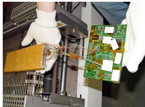
5. Carry the PCB and profiler away from the oven area, and place the shielded profiler on a flat, level surface that is unaffected by the unit's heat.
