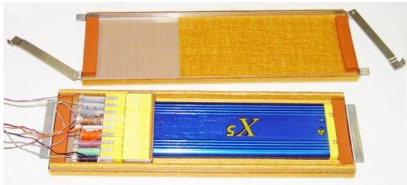
5. Carefully lift the profiler out of the shield.
