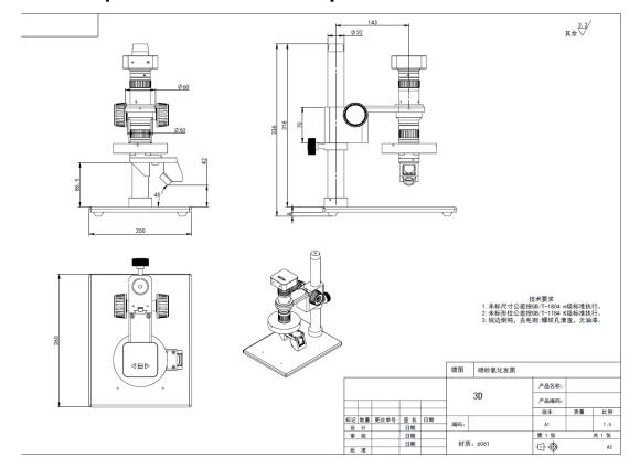
stand base 2.2D/3D rotation view 3.4 zones control LED ring light .4. Zoom body 5.CCD fine focus tube 6.HDMIcamera 7.stand post 8.Focusing holder
