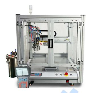
Benchtop conformal coating machine is semi-automatic conformal coating machine with transparent cover, which is a high-tech product integrating precision machinery with automatic control and precise dispensing control technology. This product has the advantages of strong function, simple programming, convenient operation and cost efficiency.
